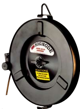
DO-3A Overhead dispenser for mill wound coils. Wall mounting bracket (WB, Part No. 002817) and ceiling bracket (CB-9, Part No. 002816) are available.
